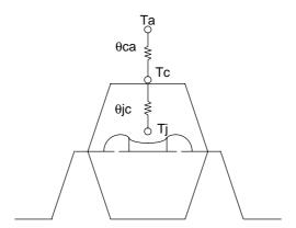
Figure 2 Thermal resistance of package
