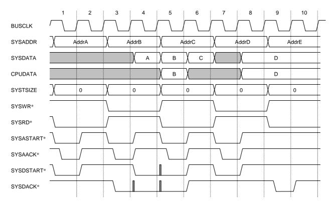
Figure 8-9. CPU Single Read-Write-Read-Write Cycles
