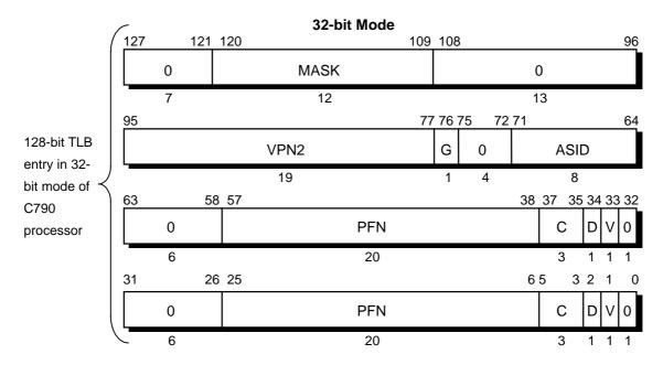
Figure 6-8. Format of a TLB Entry
