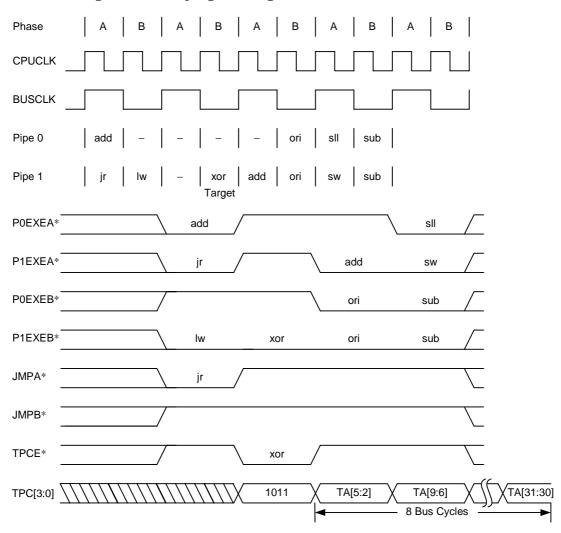
Figure 12-5. Waveform for Indirect Jump (Target in Phase B)
