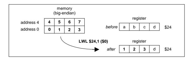
The contents of GPR rt are internally bypassed within the processor so that no NOP is needed between an immediately preceding load instruction which specifies register rt and a following LWL (or LWR) instruction which also specifies register rt.
