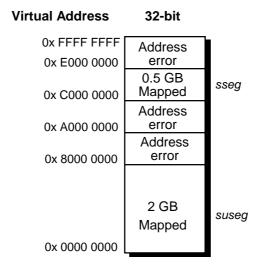
Figure 6-5. Supervisor Mode Virtual Address Space
