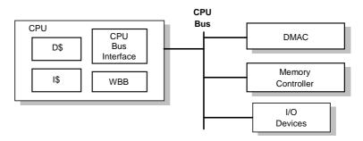
Figure 8-1. CPU Bus Architecture
