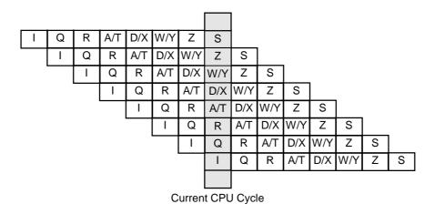
Figure 2-3. FPU Pipeline
