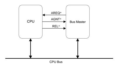
Figure 8-4. Connection of Arbitration Signals
