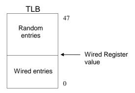
Figure 4-8. Wired Register Boundary
