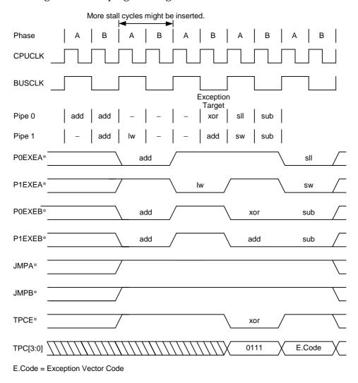
Figure 12-7. Waveform for Exception (Target in Phase B)
