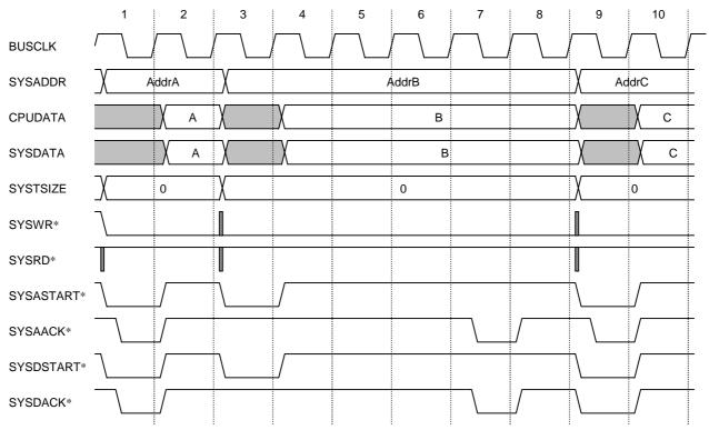
Figure 8-15. CPU Non-Pipeline Single Writes
