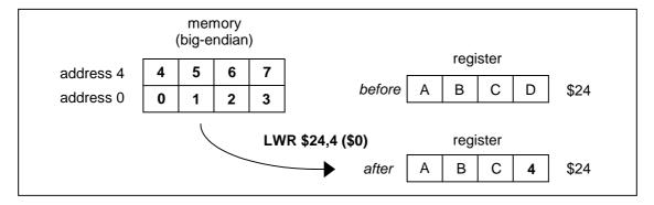
The contents of GPR rt are internally bypassed within the processor so that no NOP is needed between an immediately preceding load instruction which specifies register rt and a following LWR (or LWL) instruction which also specifies register rt.
