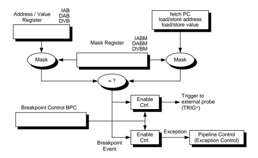
Figure 13-1. Overall Structure of Hardware Breakpoint
