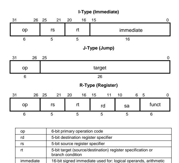
26-bit index shifted left two bits to supply the low-order 28 bits of the jump target address.
