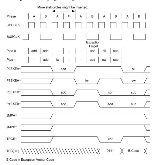
Figure 12-9. Waveform for Exception Generated by Branch or Jump Instruction
