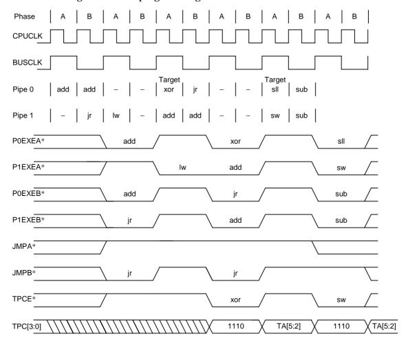
Figure 12-6. Waveform for Indirect Jump (During Target PC Output)
