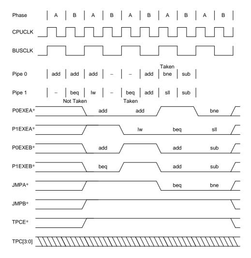
Figure 12-3. Waveform for Conditional Branch
