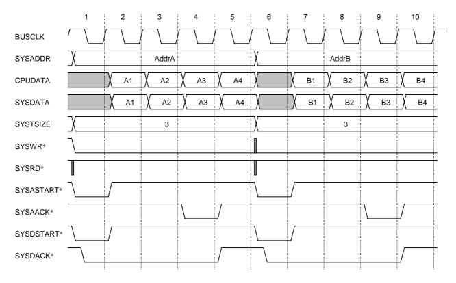
Figure 8-17. CPU Non-Pipeline Burst Writes
