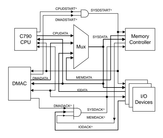
Figure 8-3. CPU Bus Data Path Connections in System
