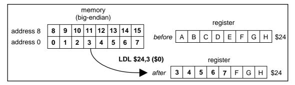
The contents of GPR rt are internally bypassed within the processor so that no NOP is needed between an immediately preceding load instruction which specifies register rt and a following LDL (or LDR) instruction which also specifies register rt.
