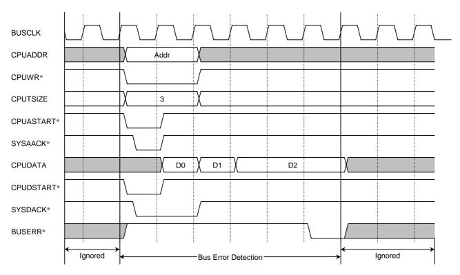
Figure 8-18. One Operation with BUSERR\* as the Last SYSDACK\*
