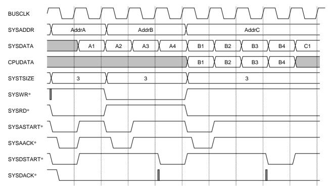
Figure 8-12. CPU Burst Read-Write Cycles
