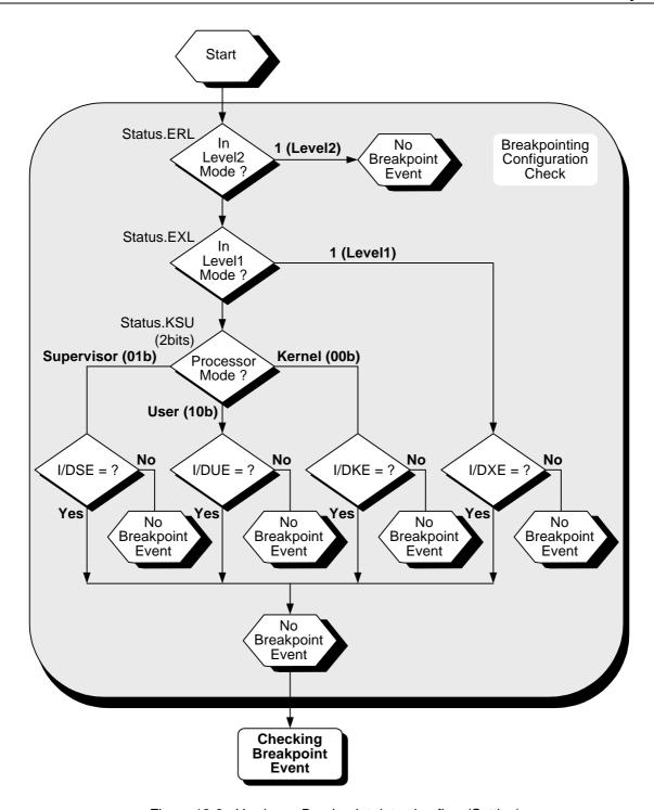
Figure 13-8. Hardware Breakpoint detection flow (Setting)
