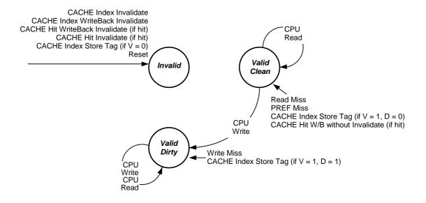
Figure 7-4. Data Cache Transition Diagram, Writeback Protocol
