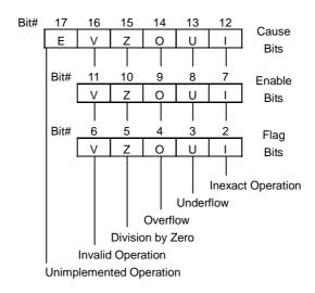
Figure 10-4. Control/Status Register Cause, Flag, and Enable Fields
