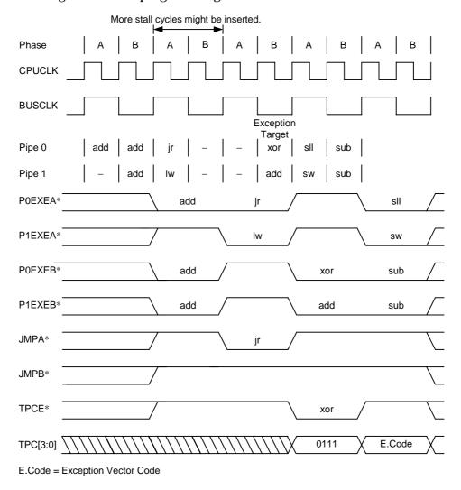
Figure 12-10. Waveform for Exception Generated by Branch Delay Slot Instruction
