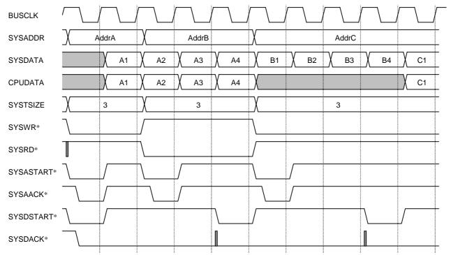
Figure 8-13. CPU Burst Write-Read Cycles
