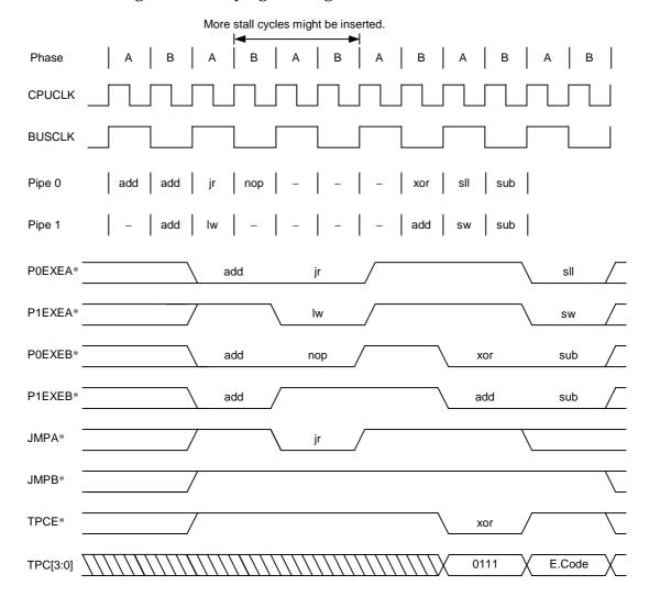
Figure 12-11. Waveform for Exception Generated by Target Instruction
