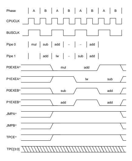
Figure 12-2. Waveform for Sequential Excecution
