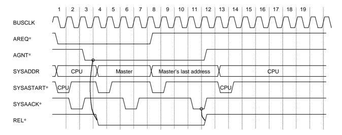
Figure 8-6. Cycle Stealing Protocol
