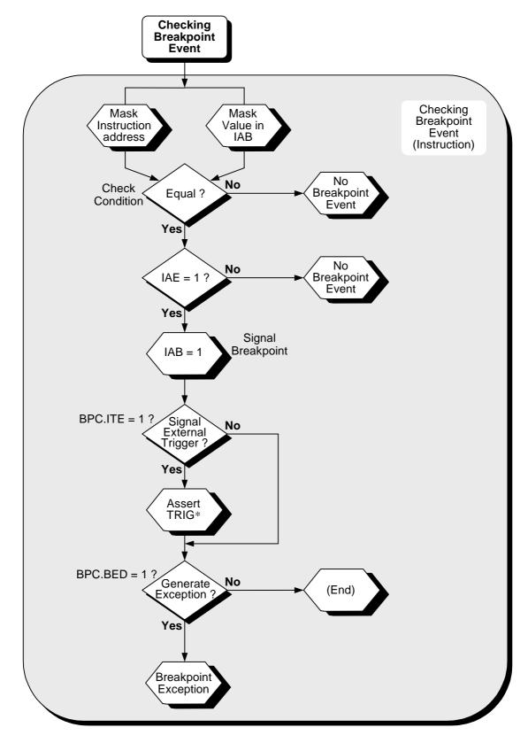
Figure 13-9. Hardware Breakpoint detection flow (IAB)
