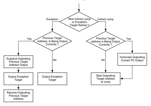
Figure 12-1. Priority of Outputting Jump or Exception Target
