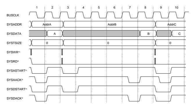
Figure 8-14. CPU Non-Pipeline Single Reads
