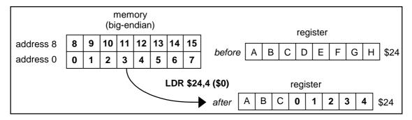
The contents of GPR rt are internally bypassed within the processor so that no NOP is needed between an immediately preceding load instruction which specifies register rt and a following LDR (or LDL) instruction which also specifies register rt.
