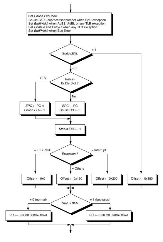
Figure 5-1. Level 1 Exception processing flowchart
