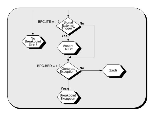
Figure 13-10. Hardware Breakpoint detection flow (IAB) (2/2)
