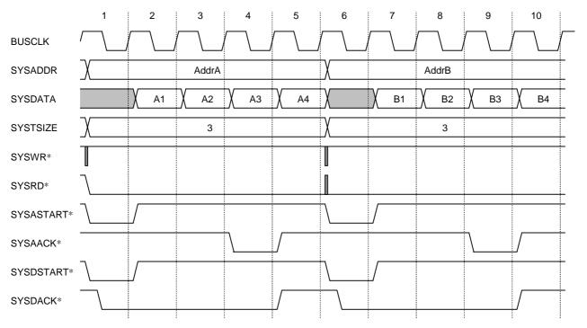
Figure 8-16. CPU Non-Pipeline Burst Reads
