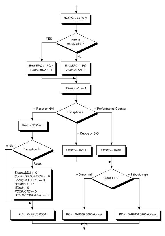
Figure 5-2. Level 2 Exception processing flowchart
