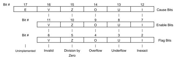
Figure 11-1. Control/Status Register Exception/Flag/Trap/Enable Bits
