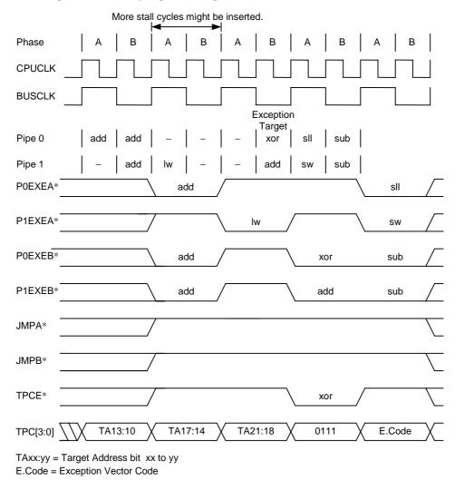
Figure 12-8. Waveform for Exception (During Target PC Output)
