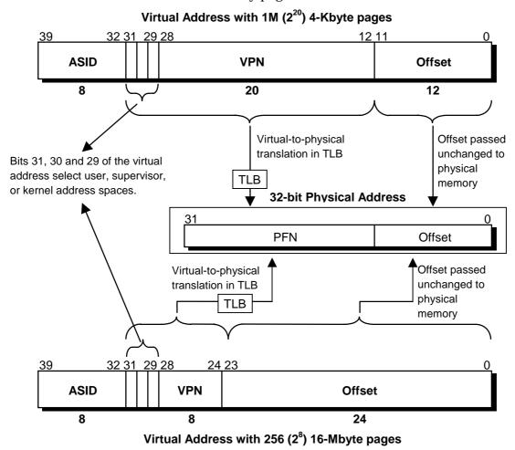
Figure 6-2. 32-bit Mode Virtual Address Translation
