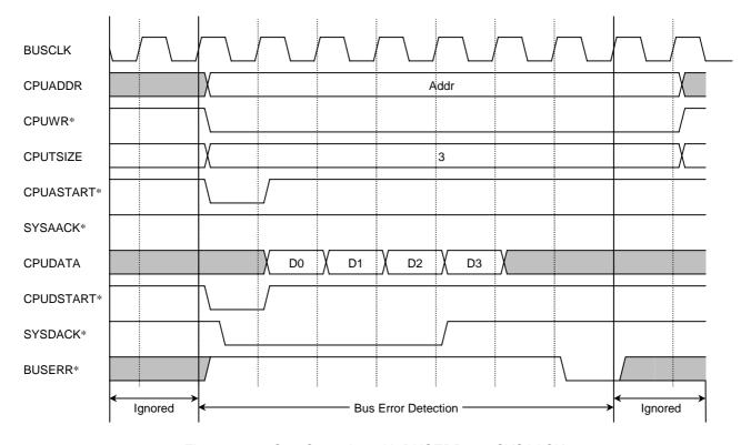
Figure 8-19. One Operation with BUSERR\* as SYSAACK\*
