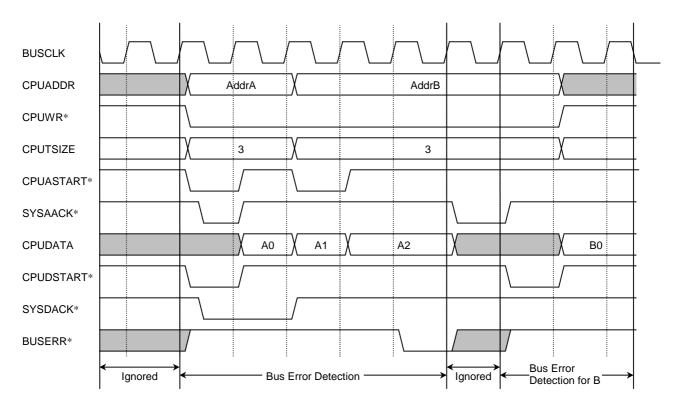
Figure 8-21. Two Operations with Bus Error as the Last SYSDACK\*
