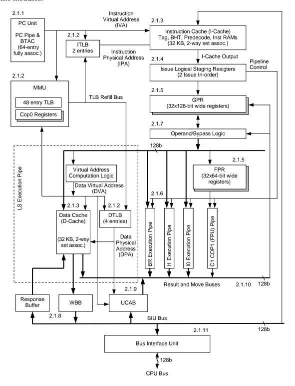
Figure 2-1. C790 Block Diagram
