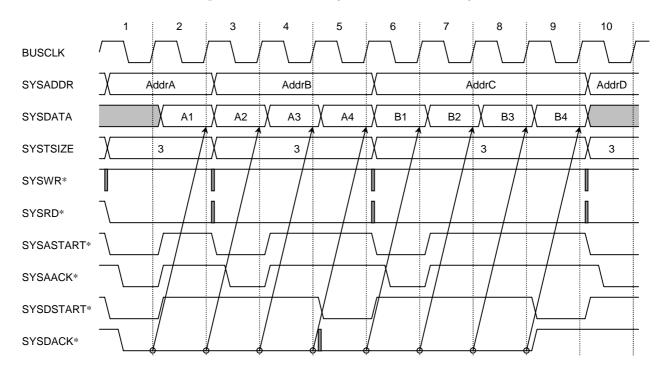
Figure 8-10. CPU Burst Reads
